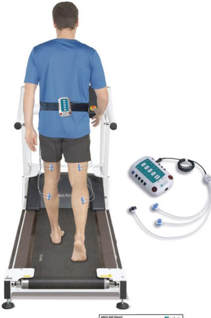
The fully synchronized zebris Myography system registers the muscle action potentials using bipolar electrodes placed on the skin surface.
