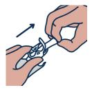
Attach the Bag Adapter to the rubber end of the CaliAdapter.
