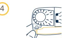
To remove the scrubber, first press down on clip at the top left-hand side of the monitor.
