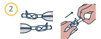
Ensure both Bag Clamps on the Quality Check Bag are closed and remove a Blue Plug from one end.
