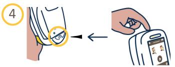
Insert the Bung into the bottom vent hole on the back of the FeNObreath<sup>™</sup> and turn the device on.
