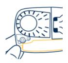
To remove the scrubber, first press down on clip at the top left-hand side of the monitor.
