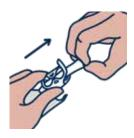
Ensure both Bag Clamps on the CaliBag® are closed and remove one Blue Plug.
