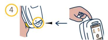
Insert the Bung into the bottom vent hole on the back of the FeNObreath™ and turn the device on.
