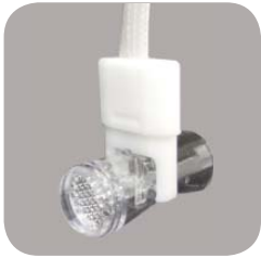
preVent flow sensor attached to umbilical
